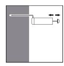
Drill hole in the substrate to the required embedment depth using the appropriate size drill bit.
