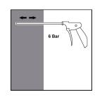
Blow twice from the back of the hole (if needed with a nozzle extension) over the whole length with oil-free compressed air (min. 6 bar at 6 m³/h). Brush twice with the specified brush size (see Table 6) by inserting the steel brush to the back of the hole (if required with an extension) in a twisting motion and remove the debris.
