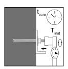
Inject the adhesive starting at the back of the hole, slowly withdrawing the mixer with each trigger pull.
