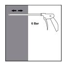
Blow twice from the back of the drilled hole with oil-free compressed air (min. 6 bar at 6 m³/h). Brush twice with the 16mm brush by inserting the brush to the back of the hole in a twisting motion and remove the debris. Blow out again with compressed air at least twice.
